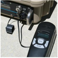
The MCD-4800 includes a standard 2-wire corded phone, however, any standard corded or cordless phone will work. The RJ-11 phone port gives a standard dial-tone and each is issued a satellite telephone number.
